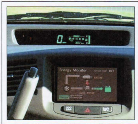
Fig. 4: Anti-reflective coatings on the VFD in this center-console application help reduce reflections from ambient light.
