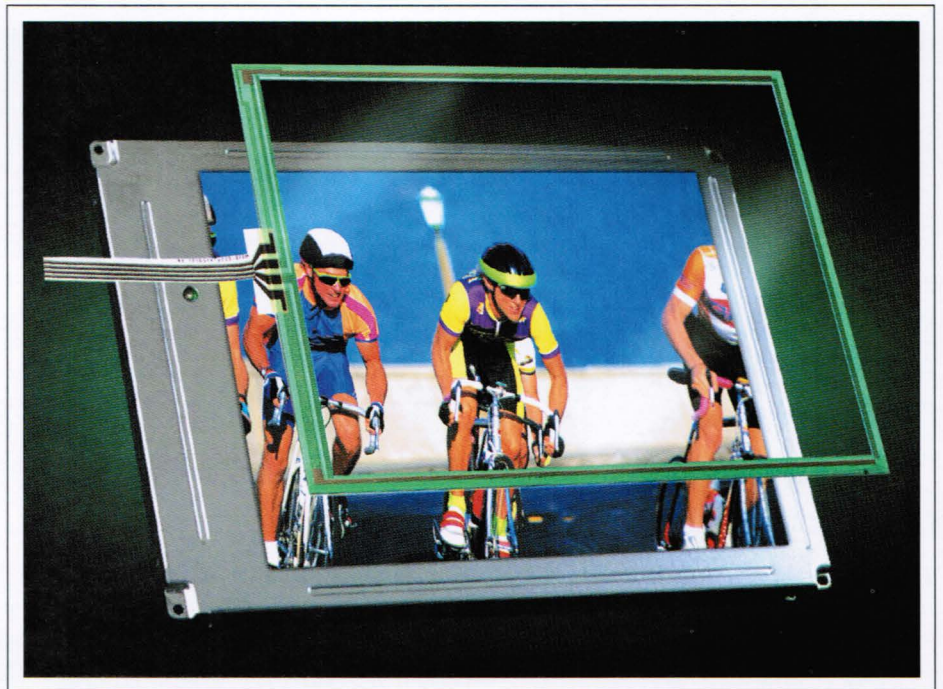
Fig. 2: The clear resistive touch panel from Fujitsu has 86% light transmission and minimal effect on the color and clarity of the Optrex 6.4-in. TFT-LCD located behind it.
