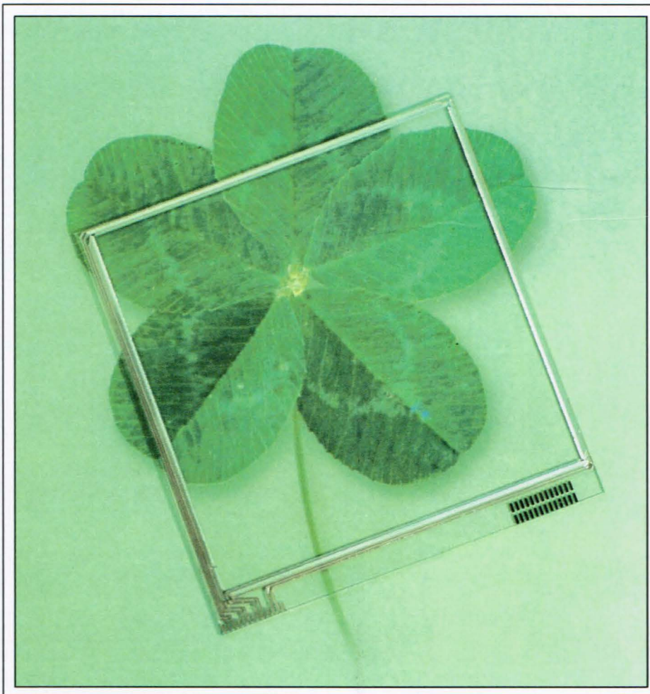
Fig. 4: Fujitsu Laboratories has recently developed miniaturized SAW technology for the portable-device market. The technology was previously suitable only for stationary large-screen applications.
