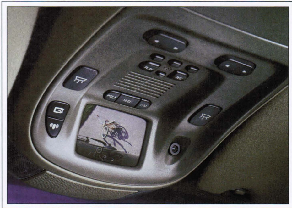
Fig. 5: An LCD panel mounted in an overhead console can provide images from a rear-facing camera to assist the driver when backing up the vehicle.
