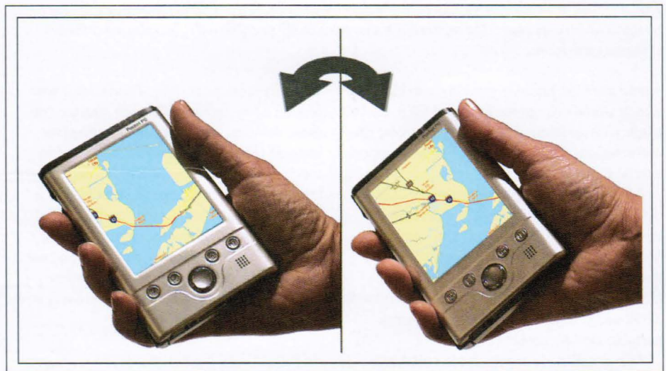
Fig. 1: Tilting a device equipped with RotoView™ scrolling technology navigates the display "window" across the image bitmap in the direction of the tilt.
